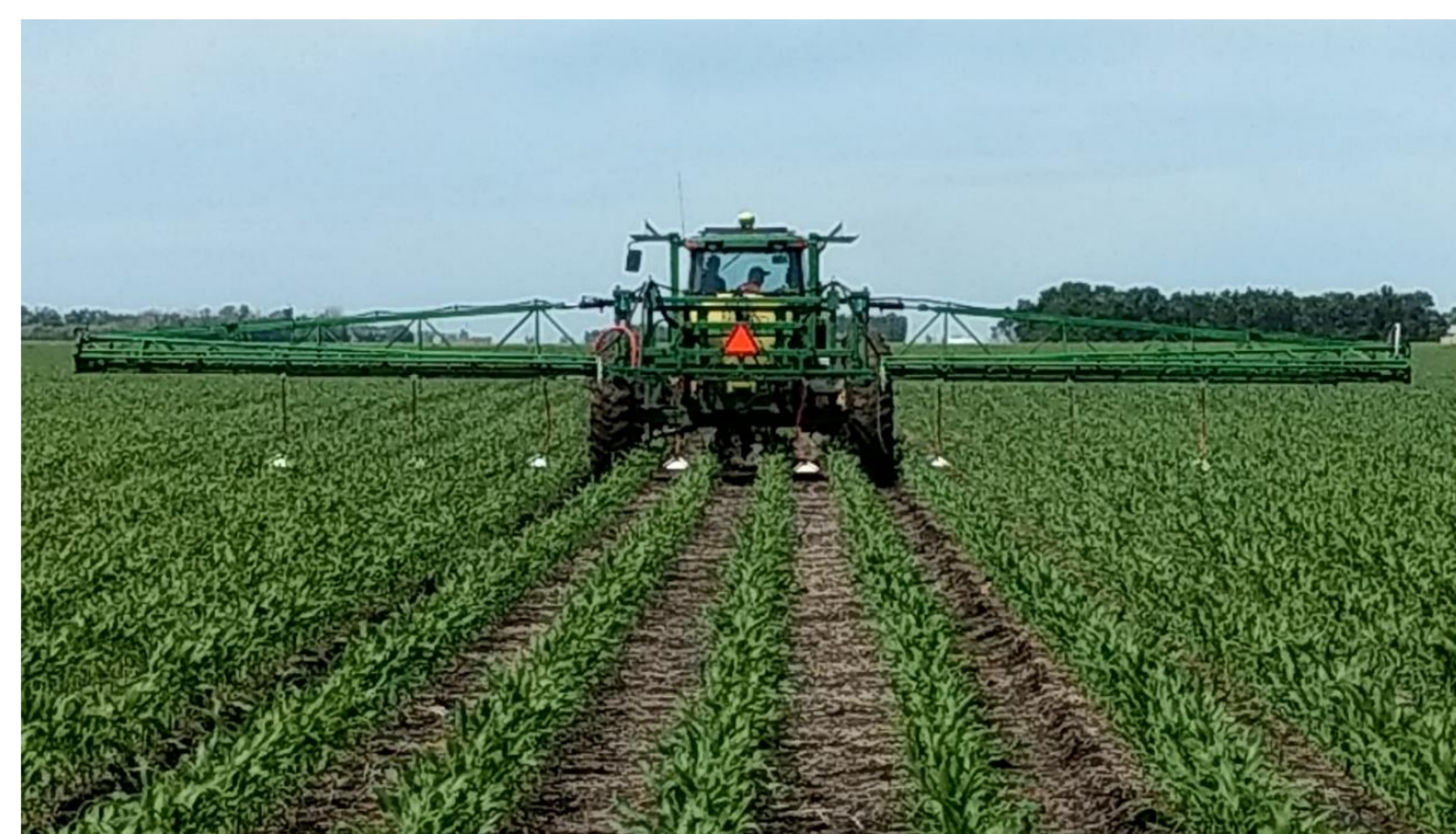
Figure 2 – Sidedress application of UAN with custom y-drop hoses
